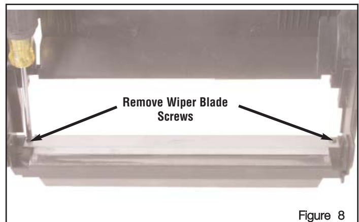
Use a Phillips Screwdriver remove the two screws from the Wiper Blade.
