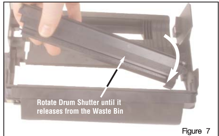
Allow removed side to fall through the opening. Then from other side rotate the Shutter until it releases from the Waste Bin.
