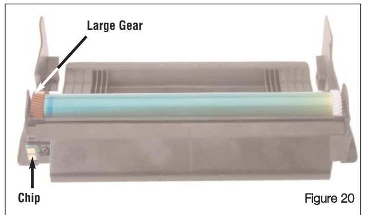
Position the Drum so that the Large Gear is on the Chip side of the Waste Bin.
